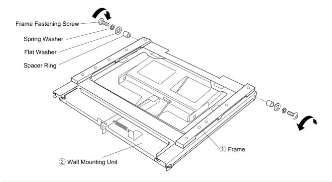
2. Push in the heads of the left and right Frame Removal Lever Screws ⓐ and lift up section ⓑ to remove the Frame ① from the Wall Mounting Unit ②.
